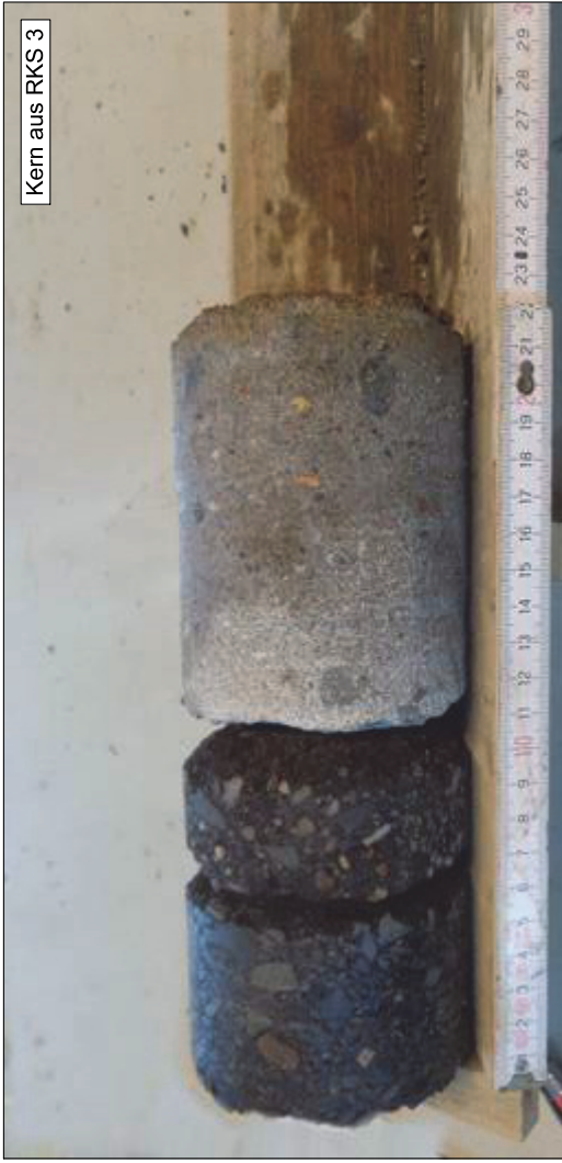
10 cm Asphalt, 12 cm Beton
